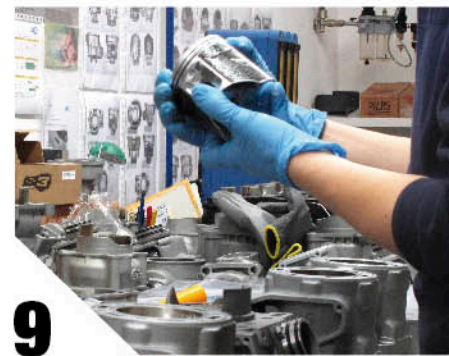
Assembling, piston + exhaust valves & packaging Control final et assemblage piston Control final y montaje del pistón
